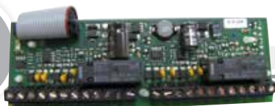
12-0109-EN: Extension card for the 2-door central unit (03-0101-EN)
